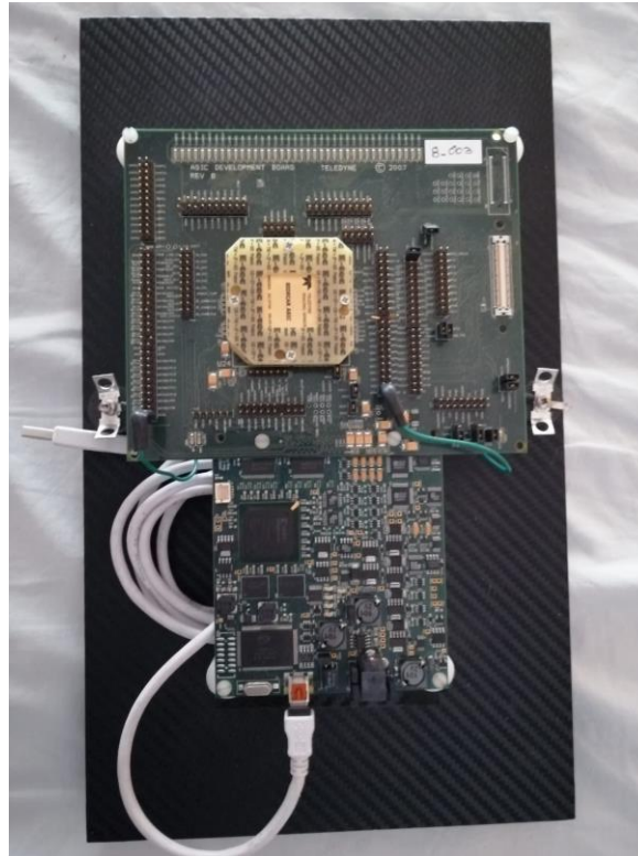
Figure 9, JADE stand-alone SCE readout system.
