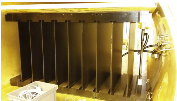
Fig. 2. The new cooling setup for controlling the fluid temperature inside the chamber.
