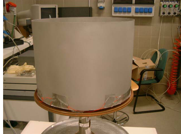
Fig. 2 Heater strips are attached to the Aluminum internal (left figure, on the 30GHz assembly) and external (right figure) structure by means of Al tape.
