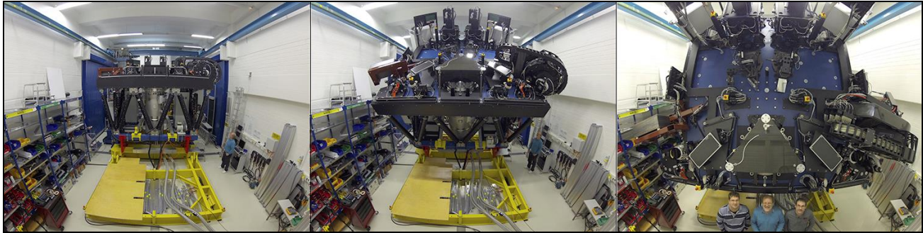
Figure 1. Flexure testing the populated LINC-NIRVANA optical bench. A large hydraulic ram tips the 10-tonne instrument from zenith to horizon, allowing assessment and calibration of flexure effects. Note the LN team members for scale.
