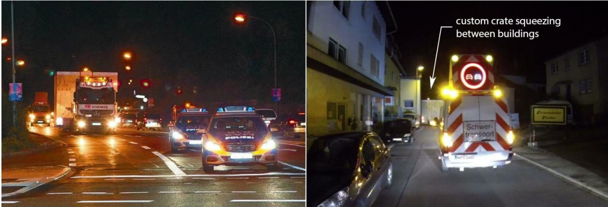
Figure 2. Some of the logistical challenges associated with transporting a large instrument through a population center. Due to its size, the LN crate required a night transport with police escort to close roads as needed (left). Some of the older surrounding villages provided interesting bottlenecks where the clearance around the crate was only a few cm (right).
