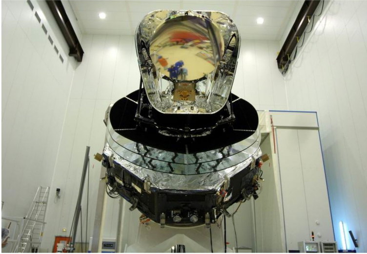
Fig. 1 the Planck Satellite, on its mounting fixture (MGSE), during the ground tests. The telescope (primary mirror) and the thermal baffle are visible in the foreground
