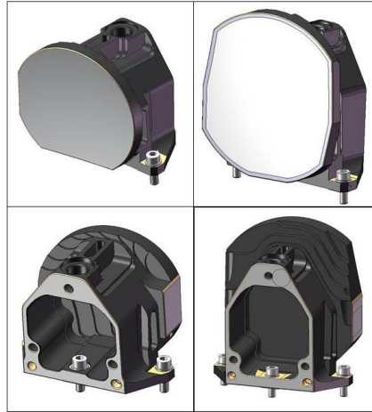
Figure 11. Pictures of parabolic mirror front and rear side (SO left, LNO right).
