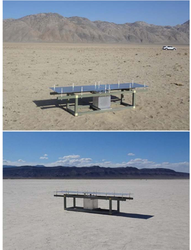
Figure 15. MIST instrument conducting test observations in Deep Springs, California (top), and in Death Valley, Nevada (bottom) in 2022 May. MIST is a single-antenna total-power radiometer without a metal ground plane. The antenna is a blade dipole of 2.4 m tip-to-tip length and the measurements span the 25–125 MHz range. These test measurements are currently being analyzed to understand the diffuse synchrotron emission in the northern hemisphere as well as the effect of the ground on the sky measurements.
