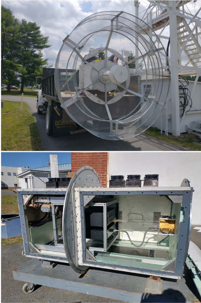
Figure 2. Some photos of the relevant instrumentation for the 310 MHz absolute map project. The top photo shows the custom high edge-taper feed, which will be mounted at the prime focus of the GBT, while the bottom photo shows the custom balanced correlation receiver mounted in a spare GBT prime focus receiver box. The 310 MHz map will have an absolutely calibrated zero-level and polarization information, which will be valuable for CMB, 21 cm, and other studies as discussed in Section 4.1.1.
