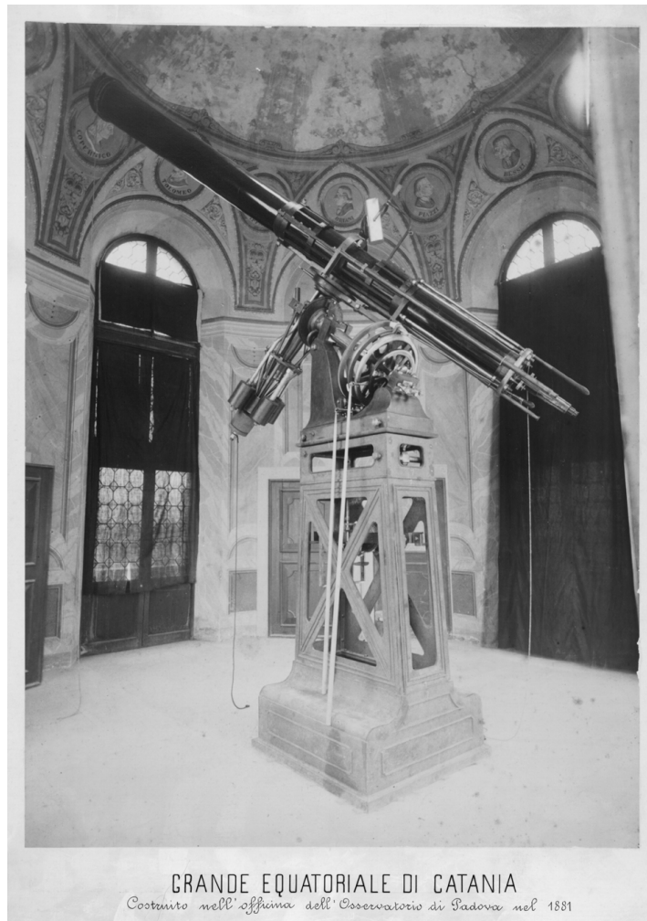
Figure 8. The Catania Observatory Merz refractor (340-mm aperture) on its equatorial mounting made by Giuseppe Cavignato at the Padova Observatory workshop (Padova Astronomical Observatory Historical Archives).
