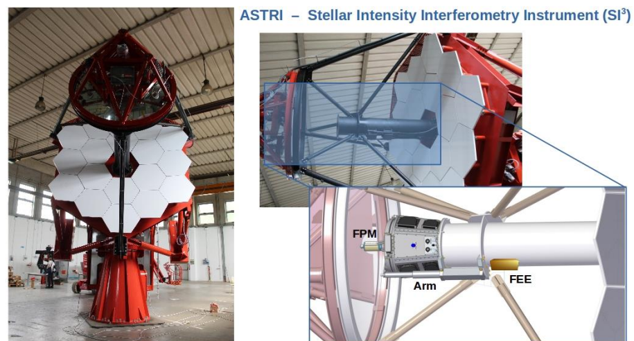
Figure 1. ASTRI telescope during factory assembly (left) and schematic view of ASTRI SI^3 (right), with the Focal Plane Module (FPM) deployed in front of the Cherenkov camera by the moveable positioning Arm and the box containing the Front-End Electronics (FEE). The Back-End Electronics (BEE) are located in the telescope cabinet and are not shown.
