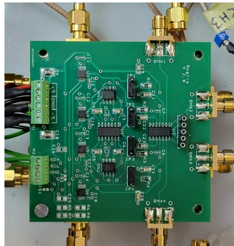
Figure 11. Threshold Generator Board as it appears mounted in the FEE box. The four DACs, recognizable in the left part of the board, are controlled by the Control Communication Unit (CCU).
