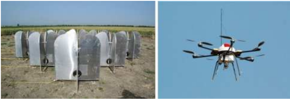
Fig. 5. Picture of MAD array (left) and the UAV equipped with RF transmitter and dipole antenna (right).
