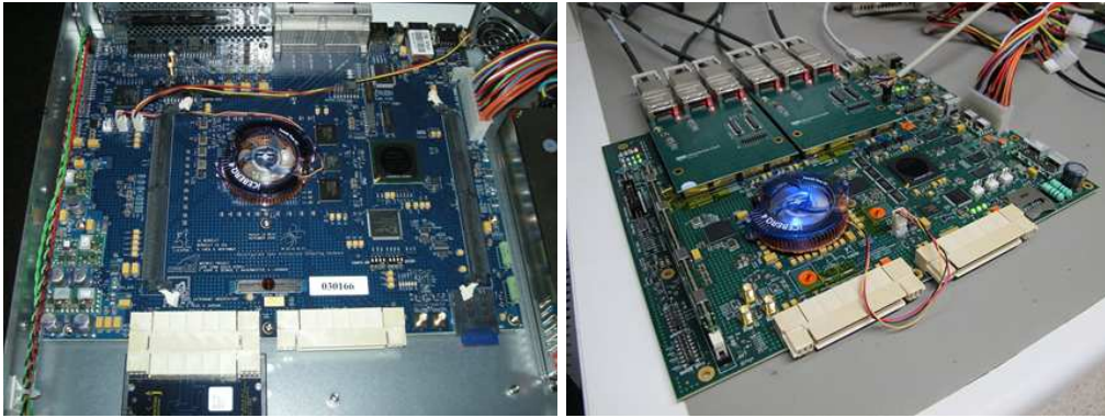
Fig. 1. ROACH1 (left) and ROACH2 (right) CASPER processing boards.
