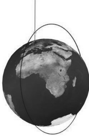
Figure 14: Intersection between the line connecting the ground station to the observed object position and the orbital plane
