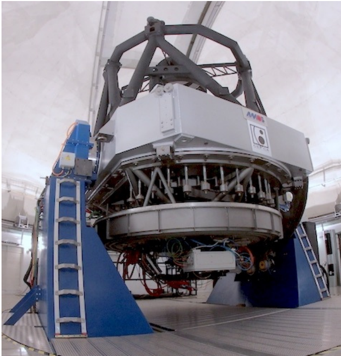
Fig. 1. View of the JST/T250 telescope at the OAJ with the JPAS-Pathfinder camera used to conduct the miniJPAS survey mounted at the Cassegrain focus.
