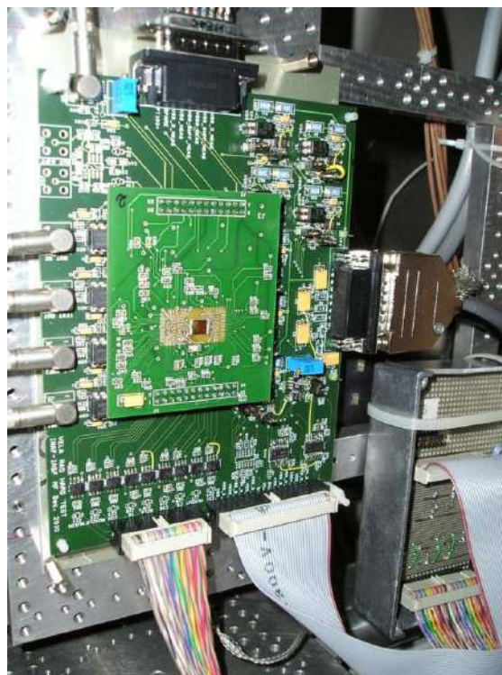
Figure 4-19 A close-up view of the the Motherboard and the Carrier PCBs. The flat cables at the bottom are used for digital signals (latch-up current triggers and LVDS VELA controls); the LEMO connectors on the left and top are VELA analog outputs and the test input respectively; the DB15 at the top of the Motherboard is used for the latch-up analog signals and the DB15 connector on the right is connected to the power supplies.
