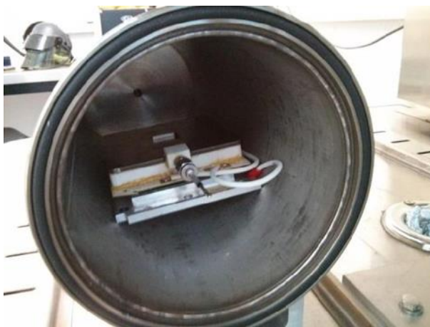
Figure 19 Picture of the GPD serial number 14 installed into the vacuum chamber (at OIA).
