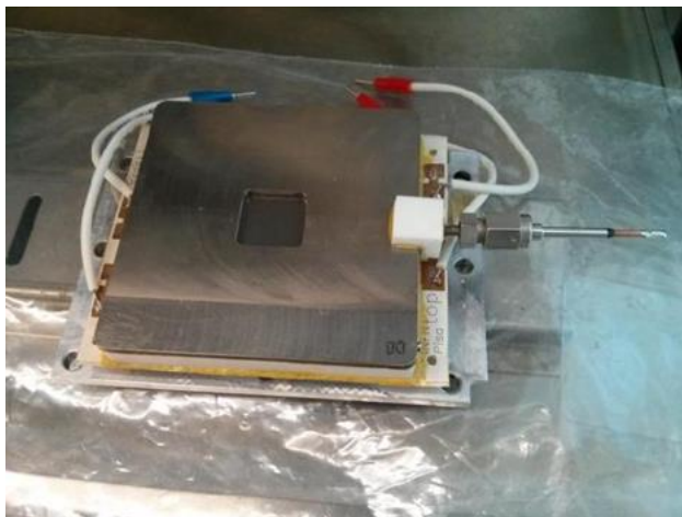
Figure 18 Picture of the GPD serial number 14, the Be window is protected by a plastic cover (to be removed during test), the gas tube and its connector is clearly visible.
