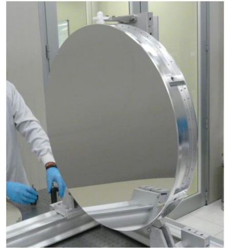
Figure 4 Prototype mirror BB700#2 under interferometric measurement in Media Lario S.r.l.
