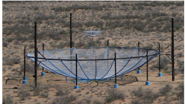
Figure 1. A single HERA antenna in the field with a cross-dipole feed surrounded by a cage hoisted to the antenna’s focal point. Image courtesy of Kathryn Rosie.
