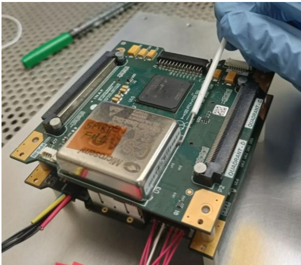
Figure 7 HERMES back-end electronics PCB
