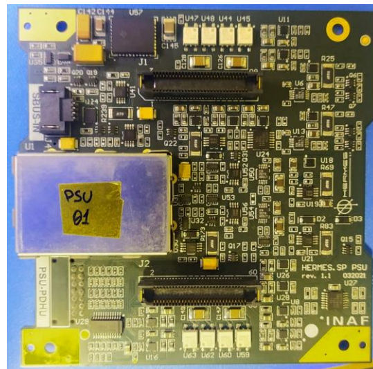
Figure 8 HERMES Pathfinder Power Supply Unit (PSU).
