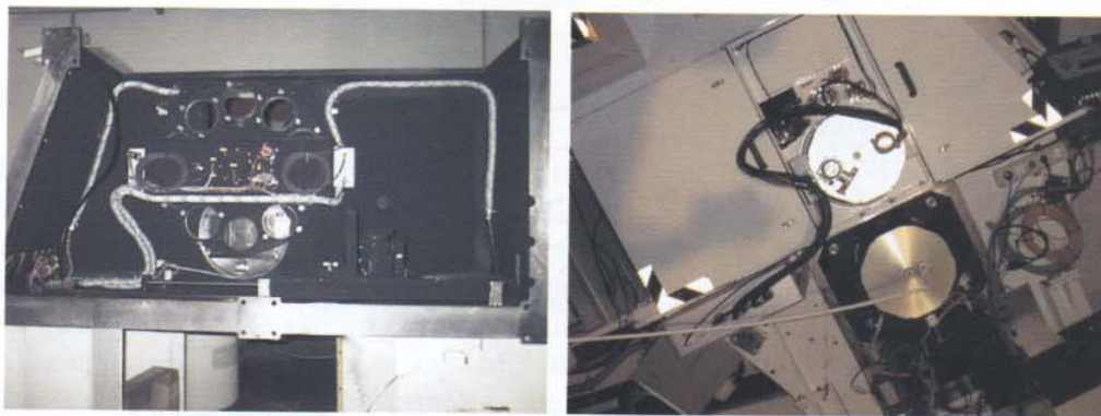
Fig. 2.2 – The OIG filter wheel inside the Nasmyth-A instrument adapter (left side). OIG and ARNICA in operation at the telescope (right side).
