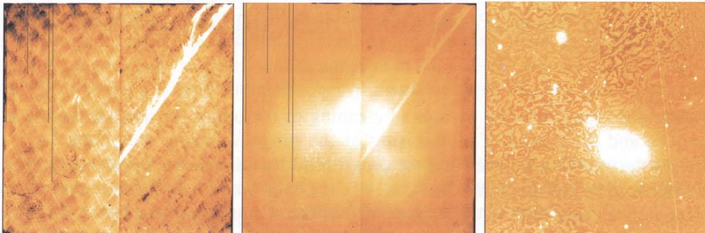
Fig. 3.2 – A series of three OIG flats made on the sky with the Johnson U, V filters and the Gunn i band filter respectively (left to right).
