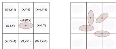
Figure 1. The C^3 sky partitioning method. The sky is partitioned in cells whose dimensions are determined by the maximum dimension that the matching regions can assume (panel a ). Each source of the second catalogue is assigned to a cell; a source and an ellipse referred to a first catalogue object can match only if the source lies within the nine cells surrounding the object (panel b ).
