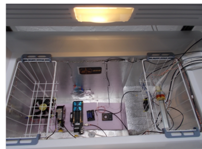
Figure 12. Cold test of motion devices
