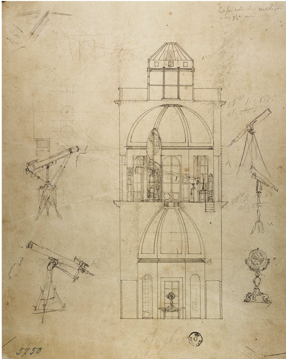
Figure 6: Vertical section of the tower of the Specola in Florence (Giuseppe Martelli 1792–1876. Gabinetto Disegni e Stampe Uffizi, Firenze, inv. 5750A). A note on the drawing refers to the lunar eclipse of 31 May 1844. Over the drawing of the upper observing room is a sketch of a large refractor, likely the Amici telescope (or its project).
