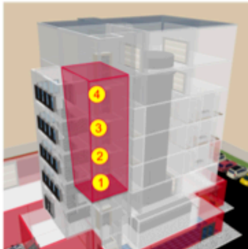
Figure 1-39. Building volume dedicated to the technical rooms.
