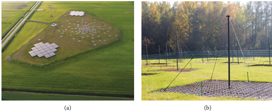
FIGURE 1: (a) A LOFAR station composed by two regular HBA arrays and the random LBA array. (b) Zoom on the individual LBA.
