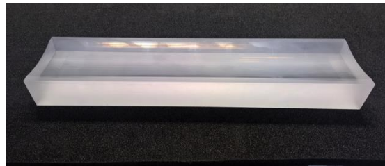
Fig. 6. Segmented parabolic mirror in fused quartz HOQ 310 being developed for the BEATRIX facility, similar to the one that will be used in VERTEX.
