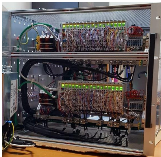
Figure 8. Beckhoff DIN rails for the DC motors control: the upper one controls the 24V DC motors; the lower one controls the 12V DC motors. Both the rails start with an EtherCAT coupler that ensure the communication with the CPU. Pull-up resistors (at the end of the rails) on limit switch signals prevent issues in case of wire breakage.
