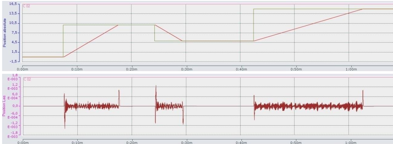
Figure 12. Details on stage positioning: target vs. actual position (top); position lag (bottom). Three consecutive positioning commands are shown: the motor works properly and always reaches the set target position (in green).
