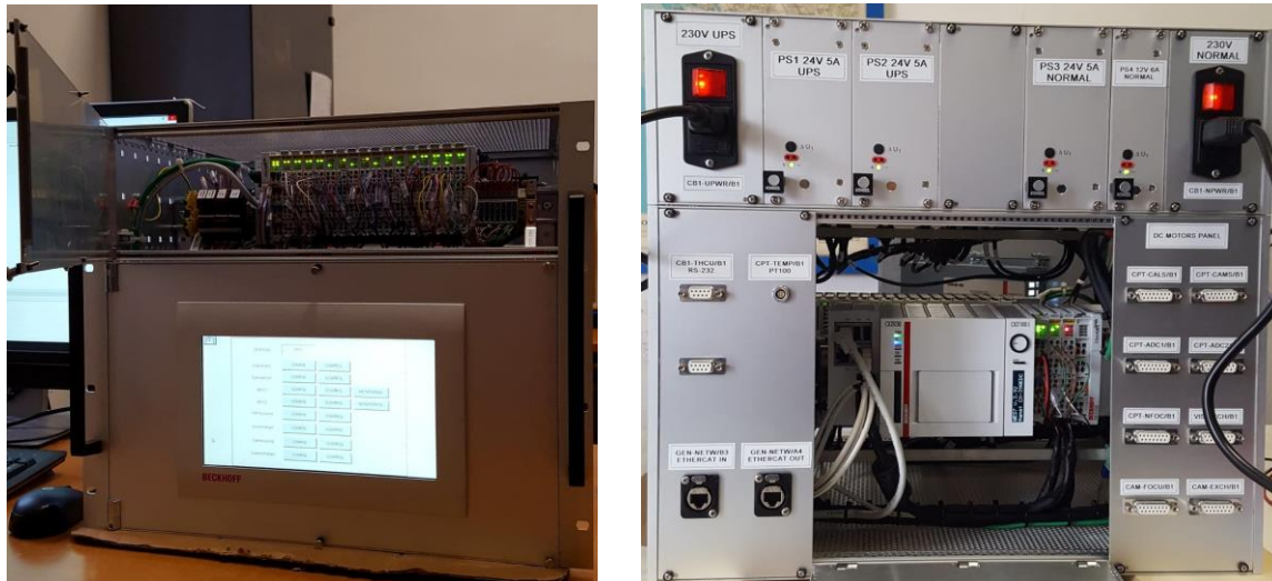
Figure 7. Front and rear view of the DC motors subrack: on the front side, the control panel allows the local control and monitoring of the instrument functions; on the back side, the Beckhoff CPU, the power supplies and all the external interfaces are accessible.
