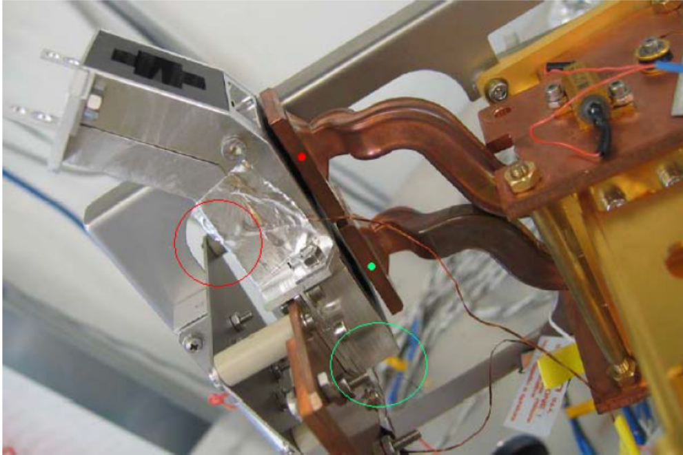
Figure 6-5 The green circle correspond to REF_TEMP and the Reference horn (green spotted) refers to channel C/D. The red circle correspond to R_MON sensor and the reference horn (red spotted) refers to channel A/B.
