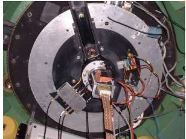
Fig. 5. The PC-ICCD mounted at the 182 cm diameter Ekar telescope. Below: observation of the Crab nebula and fourier analysis of the photons from the Crab pulsar.
