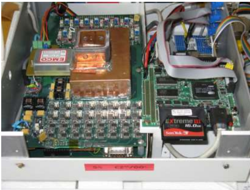
Fig. 3. The SIDERALE payload. In the foreground, on the left, the ADC board stacked on the FPGA based board, the pre-amp shield, and the detector assembly (16 pixels CZT) on top of it; on the right, the single board computer and the 16 MB Flash memory
