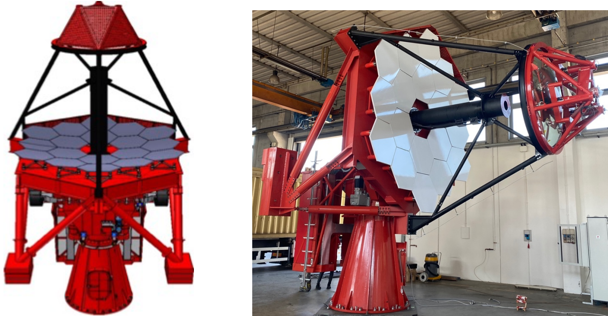
Figure 2 left: a 3-D model of the SST telescope structure; right: the first ASTRI Mini-r-ray telescope fully assembled in a warehouse in Italy before being shipped to the Tenerife Canary Island. This is also the baseline of the SST telescopes, currently under study for further possible improvements.
