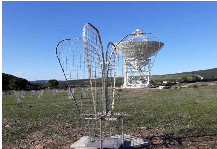
Figure 2. One of the 128 Vivaldi antennas used as front-end of our RFI monitoring system.
