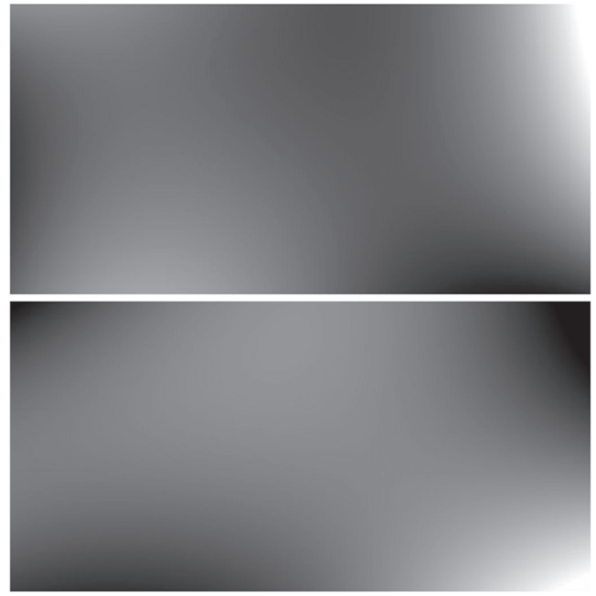
Figure 17. dx (top) and dy (bottom) that correct distortion for the Narrow camera.
