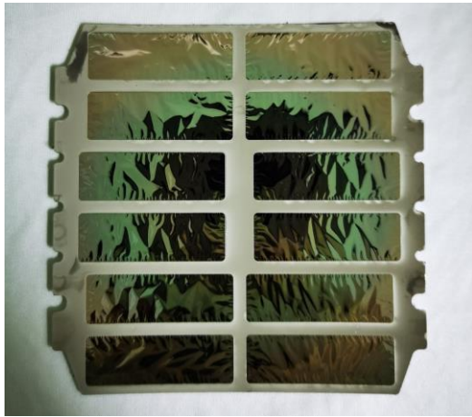
Figure 8 Left: Demonstration model of the HERMES-TP/SP filter manufactured by IHEP (Beijing). Right: Soft-X/UV/O/IR transmission of the optical filter estimated with different thickness of polyimide (1 \mu\text{m} and 2 \mu\text{m} ) and different total thickness of Al coating (200 nm and 300 nm) deposited on one or two sides of the polyimide substrate
