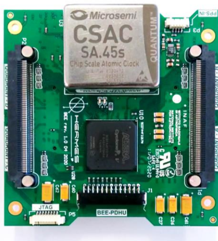
Figure 9 Left: Demonstration model of the HERMES-TP/SP back-end electronics PCB. Right: schematic block diagram of the BEE
