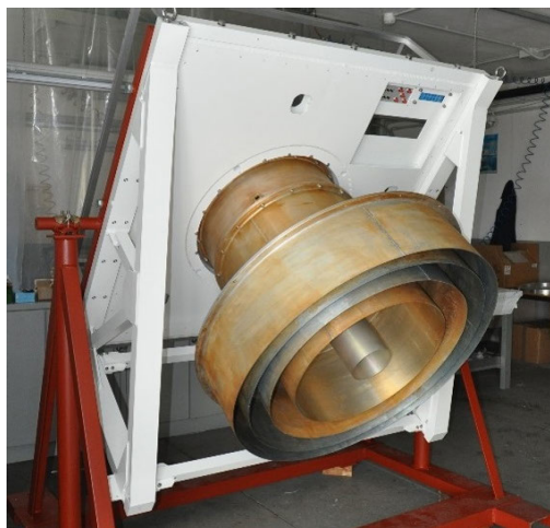
FIGURE 7. Photo of the coaxial feed.
