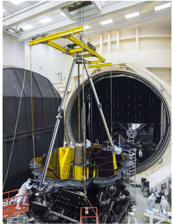
Figure 2. The JWST telescope and ISIM in preparation for the OTIS thermal vacuum test at the Johnson Space Center's historic Chamber A. (A color version of this figure is available in the online journal.)
