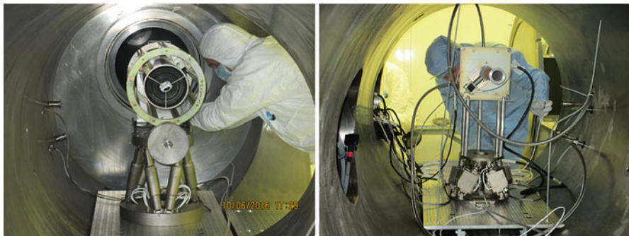
Fig. 9 (Left) The SGR ART-XC optics installed onto the hexapod inside of the vacuum chamber. (Right) The ART-XC detector placed onto an at the focus of the mirror system. (Credit: IKI)
