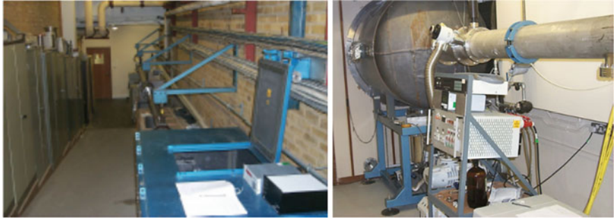
Fig. 8 (Left) The tube and the X-ray source end. (Right) The vacuum chamber from outside. (Credit: UL)
