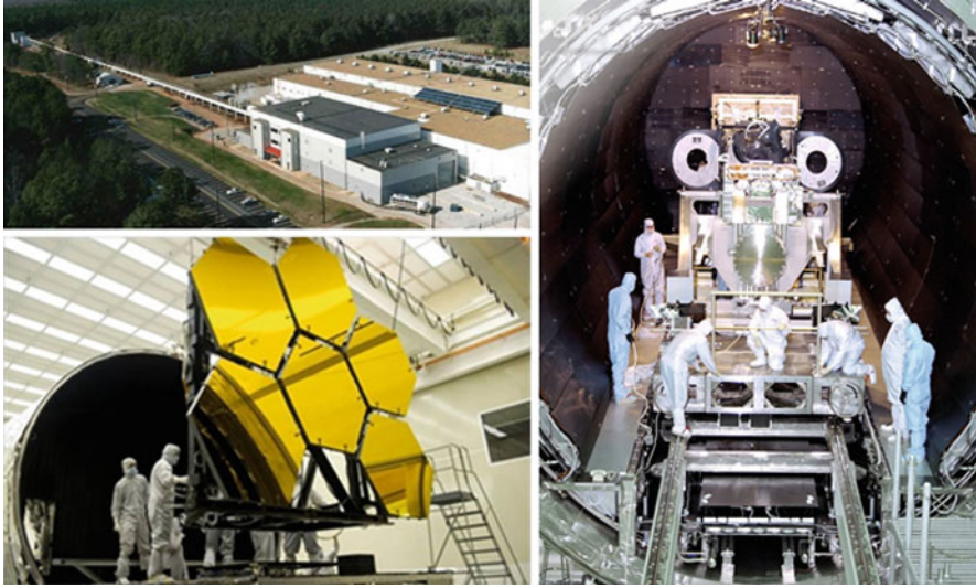
Fig. 11 (Top-Left) XRCF at MSFC. The source is located in the building on the upper-left of the image and the instrument chamber and clean room is the large building in the lower right. The beamline is 518 m long and roughly 1.5 m in diameter. (Lower-Left) Portion of the James Webb Space Telescope undergoing testing in the XRCF. (Right) The Chandra X-ray Telescope being prepped for calibration inside the facility. (Credit: NASA MSFC)
