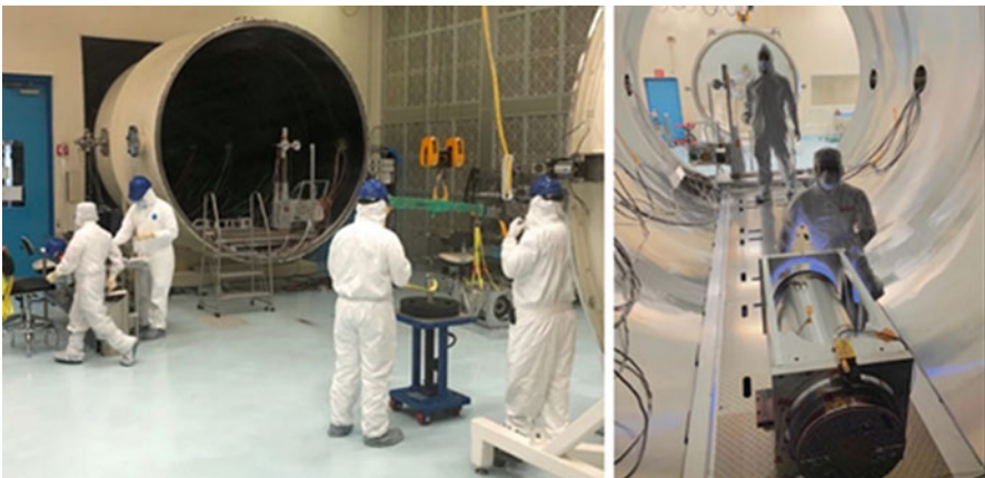
Fig. 14 (Left) Instrument chamber dome is removed for test-article integration into the chamber. The chamber is adjacent to an ISO7 (Class 10K) cleanroom. (Right) IXPE mirror module being installed inside the instrument chamber of the MSFC 100 m beamline facility. (Credit: NASA MSFC)
