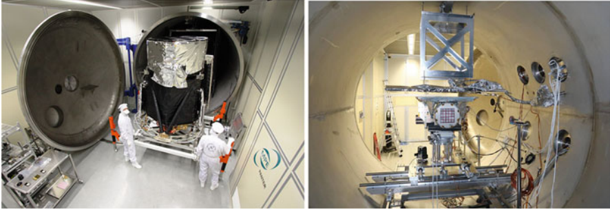
Fig. 4 End-to-end tests in PANTER. (Left) The eROSITA FM telescope entering the PANTER vacuum chamber. (Right) The SVOM-MXT-FM positioned in the PANTER vacuum chamber. (Credit: MPE/PANTER)
