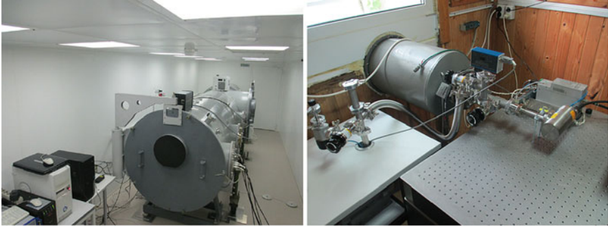
Fig. 10 (Left) The vacuum chamber positioned in a ISO-8 clean room. (Right) A micro-focus Oxford Instruments X-ray tube with a manual vacuum gate valve and a pumping unit. (Credit: IKI)
